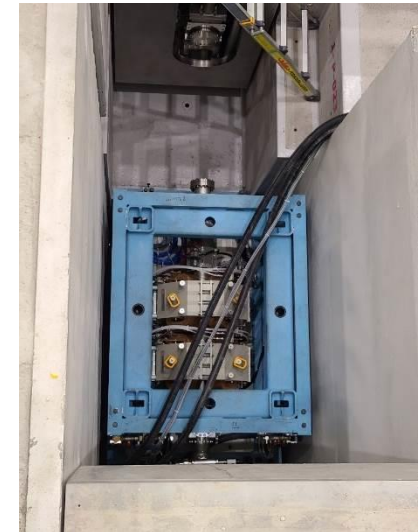
Final focusing & wobbler module in ISOL bunker (X2)
